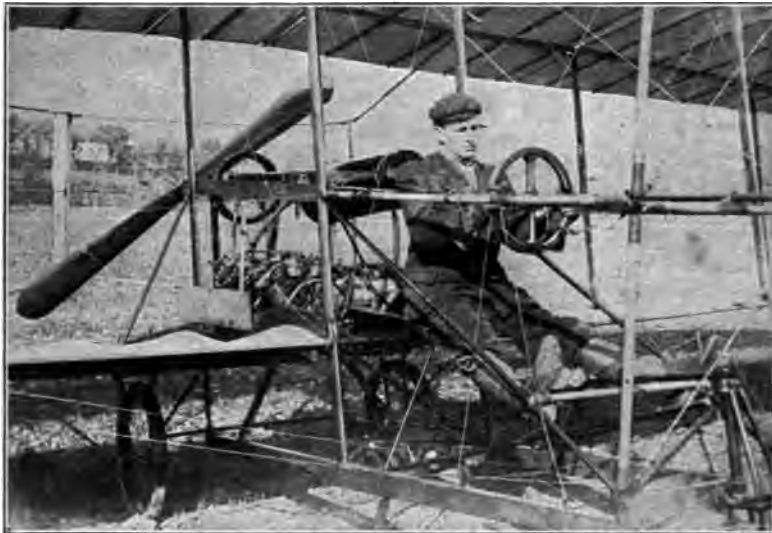
Fig. 14. View of Power Plant of Silver Dart, J. A. D. McCurdy at the Wheel
